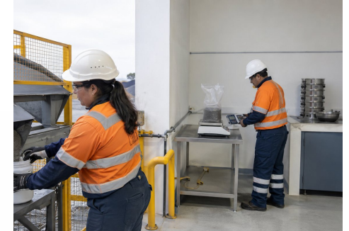
Timed sampling, weighing and sieve verification must share a traceable sample ID.
