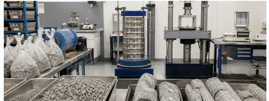
Laboratory characterization: sieve analysis, prepared rock cores and compression testing.
