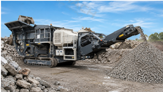
Reference visual: mobile impact crusher processing construction waste or limestone-type material.
